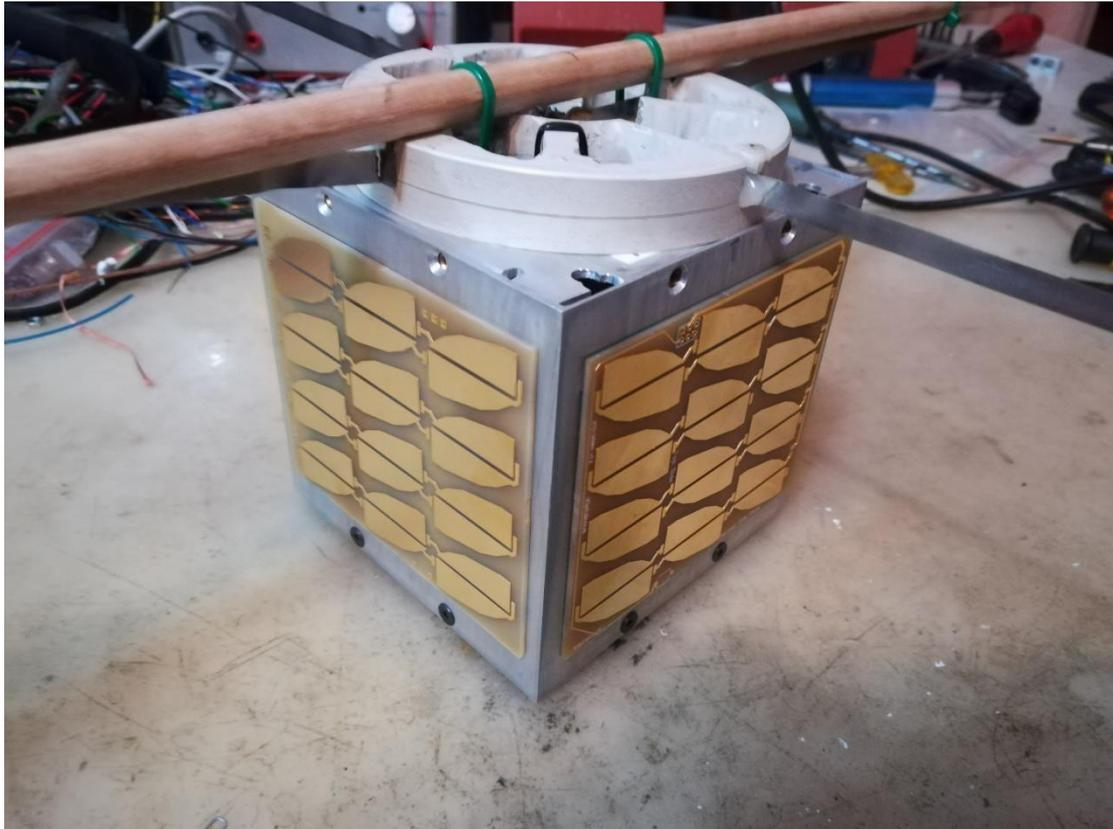
Figure 2: Prototype 2m and 70cm Crossed Dipole Antennas.
