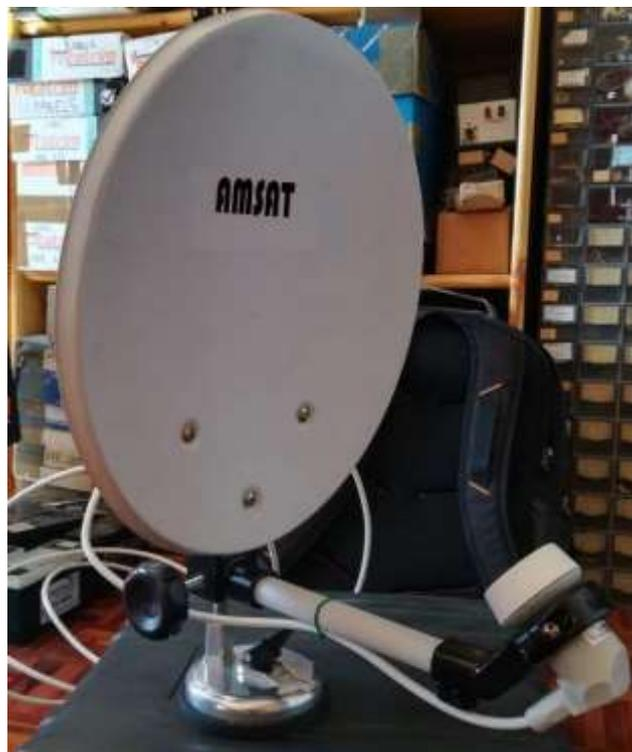
Figure 6: DSTV camping dish equipped with an ELSAT high stability Universal Ku Band LNB, ready for the 10 GHz BACAR beacons.
