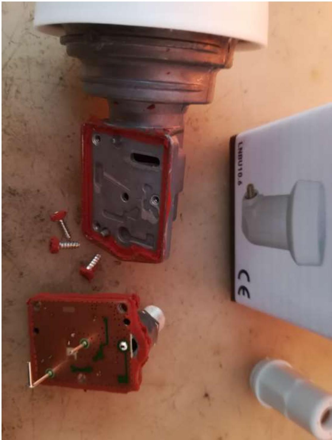
Figure 3: Disassembled, high stability, ELSAT Universal Ku-band LNB, showing a very compact PCB with the two waveguide probes.
