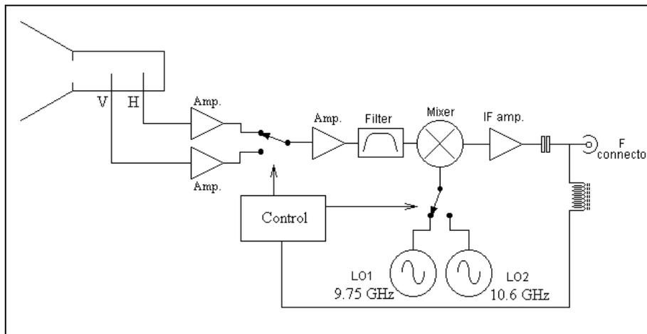
Figure 1: Universal Ku-band LNB block diagram.
