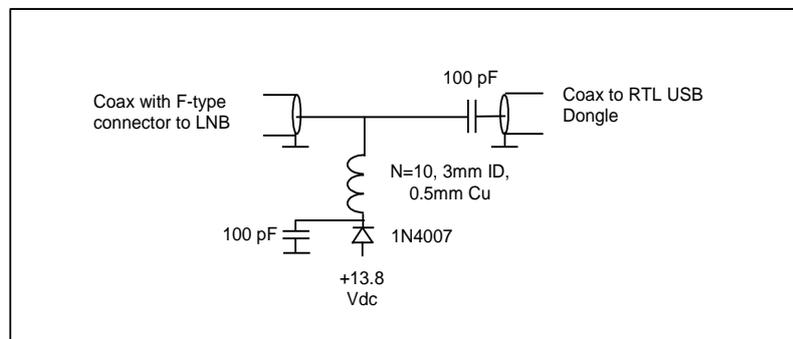
Figure 5: Bias-T or DC Injector schematic diagram.
