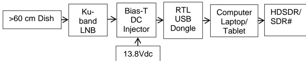
Figure 4: Possible Es'hail-2/BACAR beacon receiver chain block diagram.
